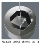
problem, because the contact surfaces that transfer the force of the tool to the screw are very narrow. The consequence: the head of the screw can be damaged, usually rounding out the recess. Hex-Plus tools have larger contact surfaces to prevent this, driving from the flats of the recess, rather than the corners. Good to know: Hex-Plus tools fit into every standard hexagon socket screw! "Take it easy" Tool Finder
