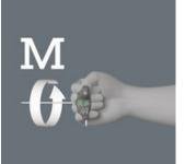
By using the blade as an extension of your lower arm you can transfer particularly high torque.
