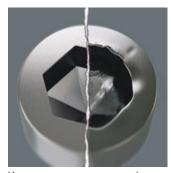
Hexagon screws can endure a problem because the contact surfaces delivering the power from conventional tool, the transferred to the screw via very small surface areas. The consequence: the screw can become damaged (rounding out). Hex-Plus tools have a greater contact surface that prevents this from happening! At the same time, as much as 20 % more torque can be applied. Good to know: Hex-Plus tools fit into every standard hexagon socket screw!
