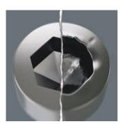
Hexagon screws can endure a problem because the contact surfaces delivering the power from the conventional tool. transferred to the screw via very small surface areas. The consequence: the screw become damaged (rounding out). Hex-Plus tools have a greater contact surface that prevents this from happening! At the same time, as much as 20 % more torque can be applied. Good to know: Hex-Plus tools fit into every standard hexagon socket screw!
