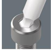
The spherical drive profile means that it is possible to swivel the axis of the tool to that of the screw, and therefore enable angled, "around-the-corner" screwdriving jobs.
