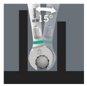
The Joker 6005 double open end wrench with its special open end design - a 7.5° offset open end and double hexagon geometry doubles the placement points at a repeated 180° rotation of the wrench around the longitudinal axis. Bolts and screw heads can be engaged every 15°. The Joker 6005 will automatically find the respective placement point after every turn.
