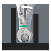
The Joker 6003 ring spanner with its special open end geometry open end offset by 7.5° and the double hexagon profile - doubles the placement possibilities when repeatedly turning the wrench 180° around the longitudinal axis. Bolts and screw heads can be "accessed" every 15°. The Joker 6003 will automatically find the respective placement point after every turn. Joker 6003: For return angles of less than 30°  $\,$
