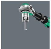
The clamping of the screw is achieved by a twin spring loaded ball retention system. The tubing is effectively protected against mechanical wear and tear by a steel ring. The holding function is especially helpful in confined, hard-to-reach spaces, where there is no room for a second hand to secure the screw.
