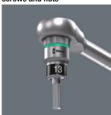
The clamping of the screw is achieved by a twin spring loaded ball retention system. The tubing is effectively protected against mechanical wear and tear by a steel ring. The holding function is especially helpful in confined, hard-to-reach spaces, where there is no room for a second hand to secure the screw.
