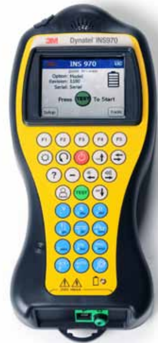
3M™ Dynatel™ Triple Play Customer Service Test Set INS970
