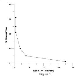
Effects of Scotch® Electrical Semi-Conducting Tape 13 on resistivity of semi-conductive cable shield.
