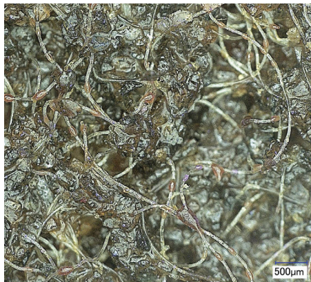
Scotch-Brite Weave, Pictured at 500 µm
