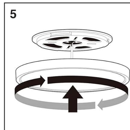
Install the lamp & rotate to lock.
