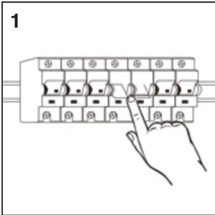
Please switch off the circuit breaker before installation & place a sticky note over it to indicate that you are working on this circuit.
