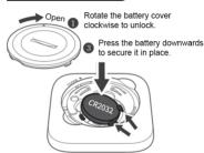
Slide battery underneath the 2 ribs located on the right.
