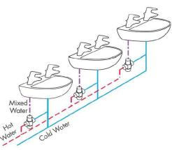
The METHVEN UK LTD range of thermostatic mixing valves MUST be installed in an accessible position to ensure that maintenance, commissioning and testing of the METHVEN UK LTD Thermostatic Mixing Valves can be undertaken easily.
