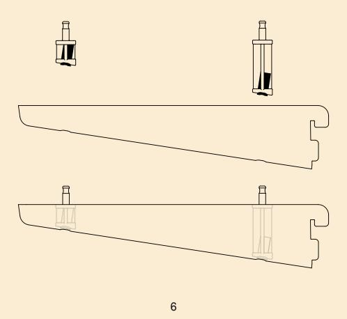
Then turn the bracket upside down, place it towards a firm support and attach the nails into the pins one at a time.
