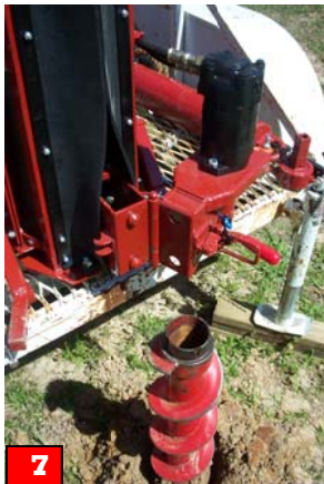
7 Remove center rod. Take soil sample as needed.
