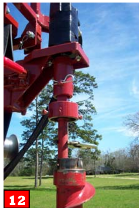
12 Raise drill head in order to remove locking pliers.
