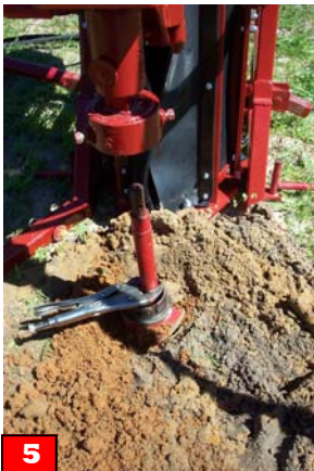
5 Remove drive cap by removing pin from drive cap, raising drill head, and removing adaptor pin.
