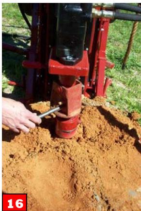
16 Use retrieval pin to connect drive cap.
