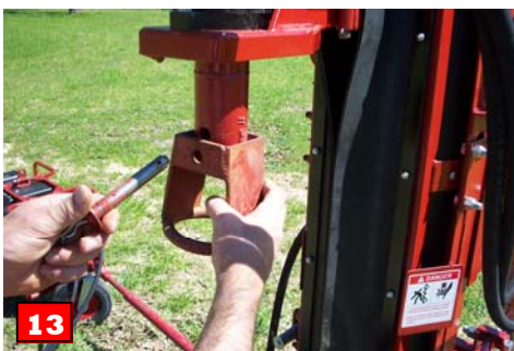
13 Connect retrieval ring to drill head with pin.
