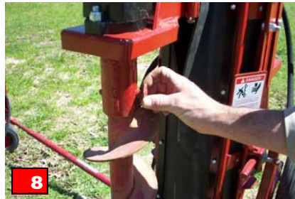
8 Lower drill head to connect extension top with pin. Repeat procedure until desired depth is reached.
