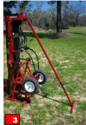
Lift back stay base. Pivot and extend back stay into position.
