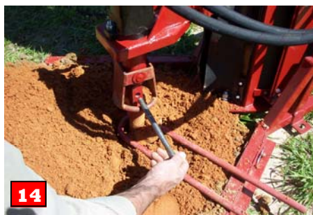
14 Lower retrieval ring over auger (extension) top and connect with pin. Remove auger fork (stop) after auger string is secured by retrieval ring.
