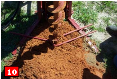
10 Lower drill head until the weight of auger string is resting on the auger fork (stop).
