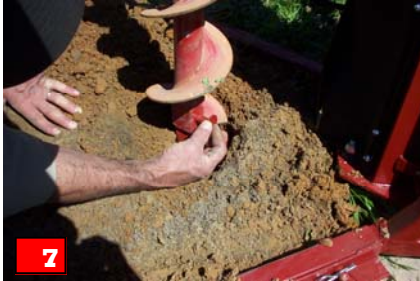
7 Raise drill head to connect extension. Connect extension bottom with
