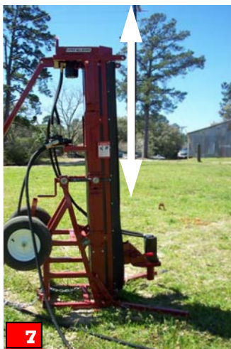
Initial angle adjustment should be slightly back from desired drilling angle.
