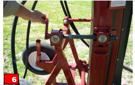
Adjust drilling angle by turning the crank handle. Tighten set bolt on side brace after adjustment.
