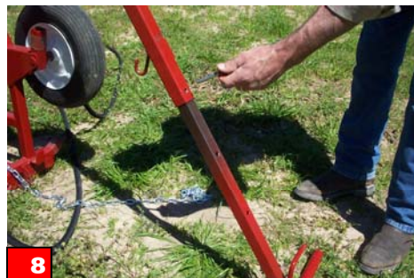
Pin the center (third) hole (or the nearest hole which allow clearance from obstructions) of back stay.
