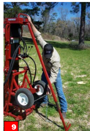
Push the top of the mast forward and hook a link in the chain to the back stay. Pull back on back stay to remove slack in chain.
