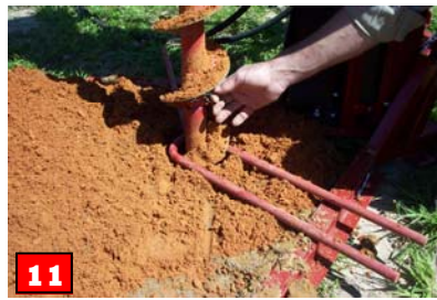
11 Disconnect extension bottom by removing pin.
