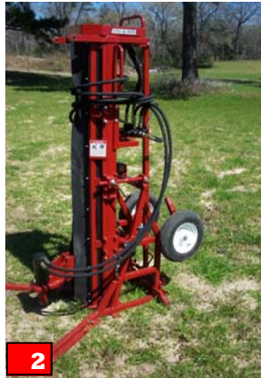
Stand drill upright, into desired position to drill hole.
