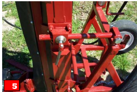
Loosen set bolt on side brace.
