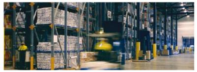
Drive-In pallet racking is the lowest cost and most popular form of high density pallet storage. Drive-In racking provides excellent storage capacity in applications where there is a large quantity of pallets for each SKU. It is ideal for many industry sectors including general manufacturing, food and beverage as well as the cold storage industry.
