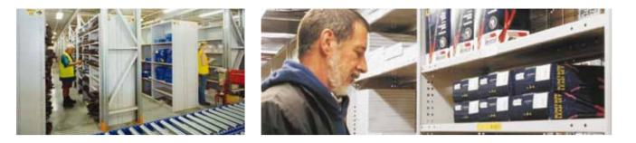
Steel shelving is the lowest cost and most frequently used storage solution for slow moving goods, parts and files.
