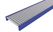
The 24V dc accumulation conveyor offers true 'zero pressure' accumulation. A motorised roller ensures products are held captive within each accumulation 'zone'. The conveyor requires no other drive devices or controls. Start/Stop control is performed automatically and without the need for additional air-operated devices such as pneumatic roller brakes and case stops.
