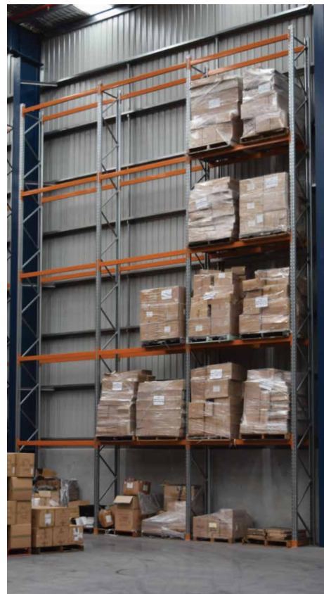
Left: Structural columns are integrated within the racks. Right: Custom-width bays of racking enable space between structural columns to be utilised.
