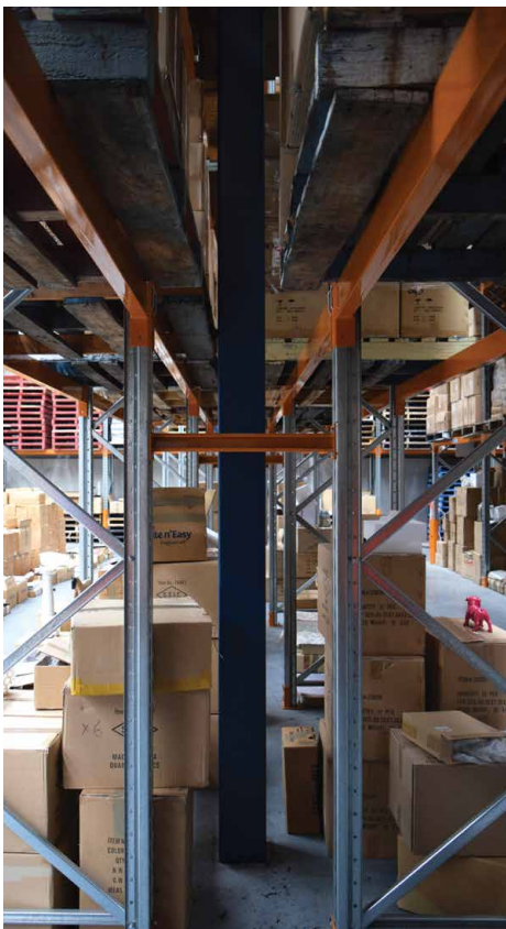
Left: Structural columns are integrated within the racks. Right: Custom-width bays of racking enable space between structural columns to be utilised.
