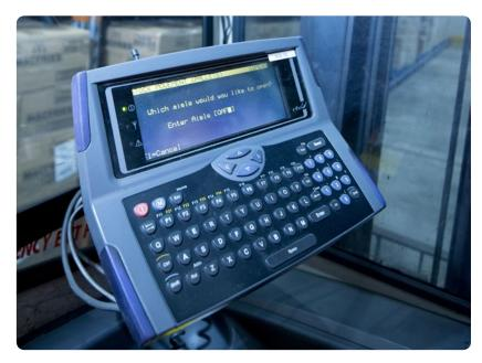
the new aisle where required. The process of opening aisles can also be automated through the user's WMS, saving further operator time, with the aisle already opening by the time the forklift driver arrives at the location.
