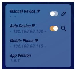
For the WS66i network connection, you can either choose the Manual setup, or the Auto Scan option
