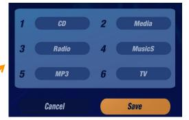
When the WS66i installed, the sources are numbered. You can custom (e.g. CD, MP3, TV, Stream, etc) in the blue oval boxes, enter the names for the source, and click Save
