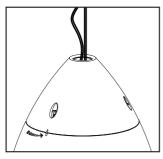
8. Place cover plate on the speaker and slightly rotate it until alignment indicators meet.
