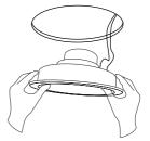
Note: The flange of the speaker is designed to flex and conform to any small imperfections in the wall surface. Tighten the 6 screws on the front of the baffle only enough to make the flange become snug against the ceiling or wall. As you tighten the screws, the feet will automatically flip into an outward position, thereby clamping the drywall between the feet and the flange.
