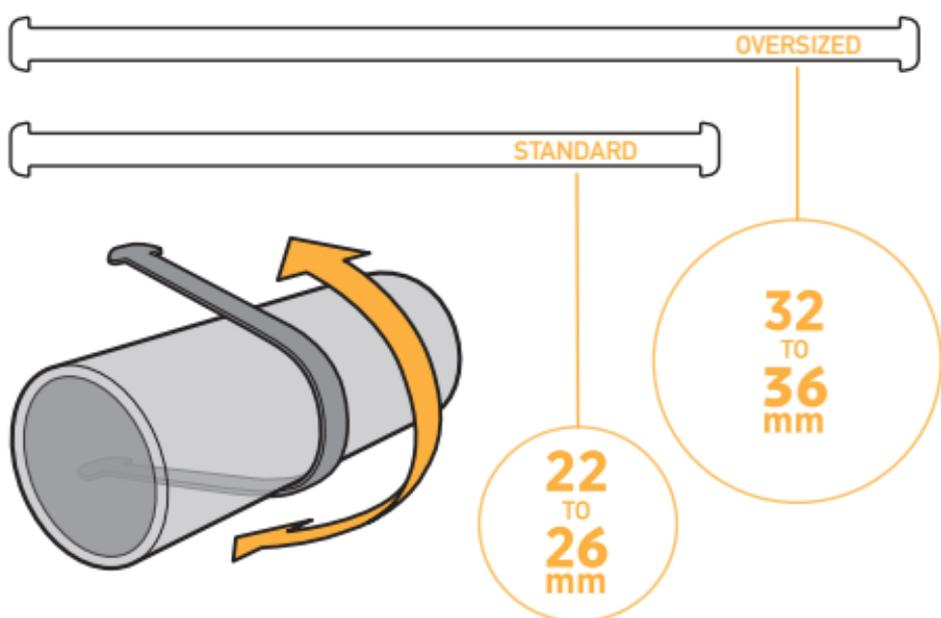
**2** INSERT BAND ENDS INTO SLOTS INSIDE BELL AND RELEASE, ALLOWING BAND TO LOCK IN PLACE.
