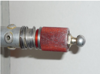
The Uerlings sleeve and similar threaded sleeve used on LS gliders rotate or unscrew over the coupling and cannot be moved into position if the ball and socket are only partially engaged
