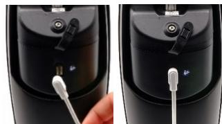
Disconnecting the charger from the prosthesis or mains will be confirmed by a vibration. Reclose the cap properly, since there is a risk of magnetization of metal particles, which would disrupt the connector's connection.
