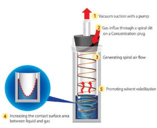
Vortex-assisted Vortex Concentration increases the contact surface area between liquid and gas, which promotes the speed of concentration.
