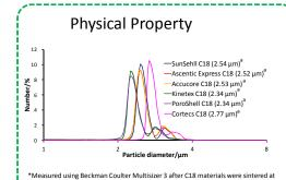
600 degree Celsius for 8 hours. The measured value of each sintered core shell silica is considered to be different from that of the original core shell silica
