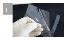
Peel off the separation film using a slit to expose the adhesive side of RAPID CRS.
