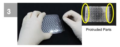
Cut both protruded parts along the dotted line while pulling them upwards, then please hold the plate with other hand, otherwise it is difficult to cut well.
