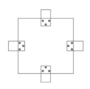
1. PLACE BRACKETS IN TABLE BASE GROOVES AND SCREW INTO PLACE.
