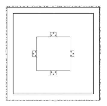
2. PLACE TABLE TOP FACE DOWN AND ALIGN TABLE BASE WITH BRACKETS TO UNDERSIDE OF TABLE TOP. SCREW INTO PLACE. .
