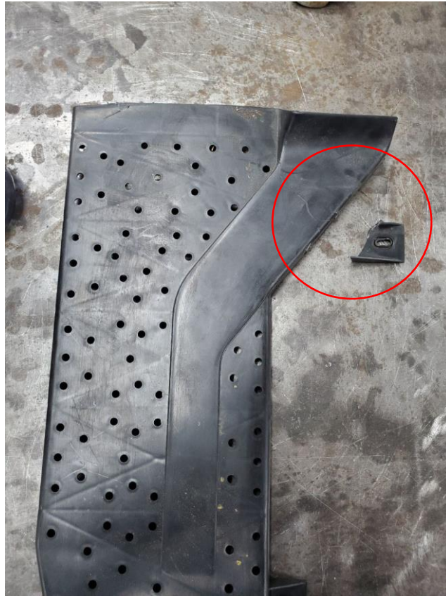
Utilizing shears or a razor blade, carefully remove rearmost mounting tab.
