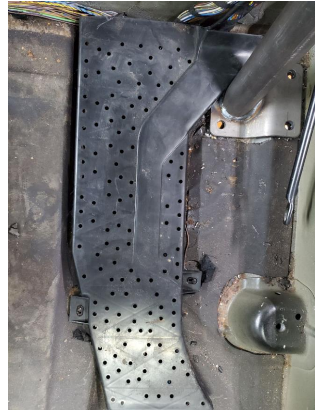
Interference removed, once installed wire cover can lay over rollbar baseplate.
