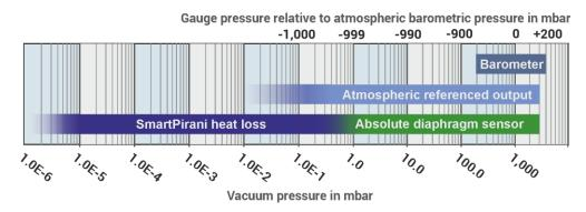
A Load-lock is a vacuum chamber used for loading devices like semiconductor wafers from the ambient air pressure to the vacuum processing chamber. The Load-lock is typically cycled between atmospheric barometric ambient pressure and an adequate vacuum pressure required to transfer the wafers to the processing vacuum chamber. Accurate control of pressure in the load-lock vacuum chamber is critically important to prevent ambient air and particulate contamination of the load-lock and wafers.
