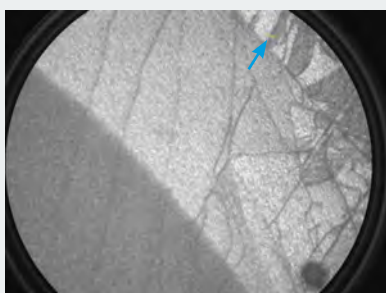
Bright-field LEEM image of MoS 2 on SiO 2 on Si taken (courtesy of J. Jobst). 7 μm field of view
