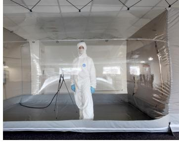
A ground sheet made from anti-static reinforced Tryoll to create a tough durable base unit. The one-piece top tent comprises two compartments; an entry airlock/ gowning room and the main work cabin which is contained within a high quality PVC envelope, making good use of ambient lighting. Positive pressure is provided by fan/filter units mounted at work station level on the work cabin gable wall.
