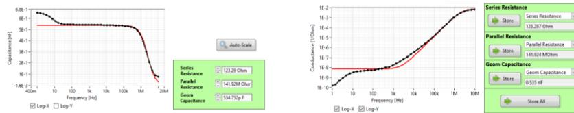
A very reliable method to extract the series resistance and the geometric capacitance from impedance spectroscopy data.
