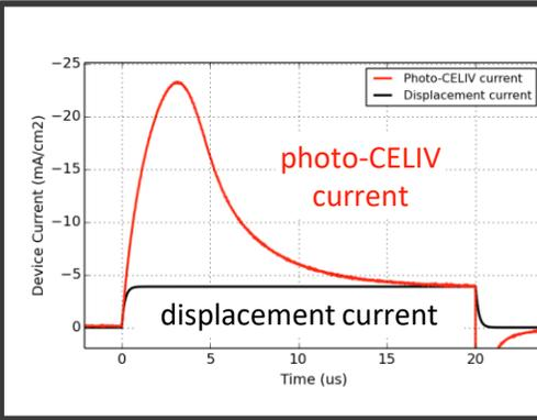
RC-effects are superimposed on the device current and can significantly disturb transient experiments.
