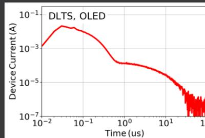
Deep-level transient spectroscopy (DLTS) is a measurement to characterize traps inside a diode.
