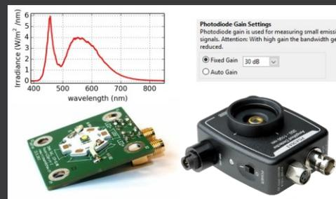
**SOLAR CELLS:** the main hardware is equipped with a suitable LED illumination system. A multi-LED board can be employed for External Quantum Efficiency (EQE) measurements.
