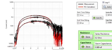
Determine the permittivity/capacitance and the series resistance from a small voltage pulse in reverse.
