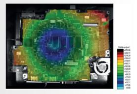
In-plane deformation field with microDAC® TL
