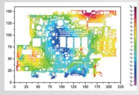
Out-of-plane deformation field (Warpage) with chromatic sensor
