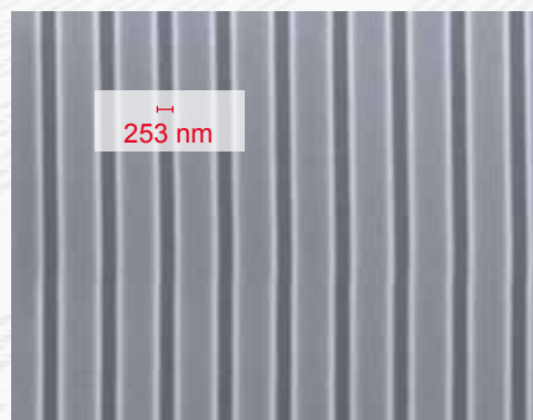
Minimum feature size: 300 nm - or even less. The image shows the result of a high-resolution test exposure with a nominal linewidth of 250 nm!
