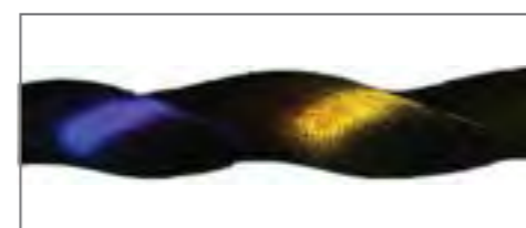
Pac-Dent R/D lab test shows how different heat treatments affects a file's surface color. Different levels of heat resulted in blue, purple, and gold colors.
