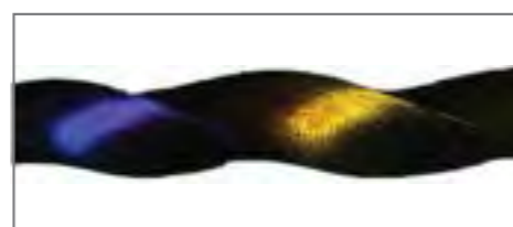
Pac-Dent R/D lab test shows how different heat treatments affects a file's surface color. Different levels of heat resulted in blue, purple, and gold colors.
