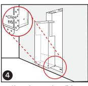
Hover door panel parallel to base until clips are aligned. Drop-in to engage.
