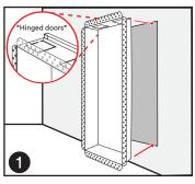
Dry fit body into vent opening. Hinged doors should be on the top.
