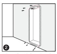
Ensure flange is flat to the wall. Use screws to fasten as needed.
