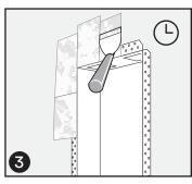
Tape and mud drywall compound to cover flange. Allow to dry. Sand and repeat as needed.
