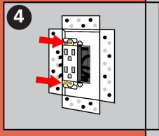
Fasten the outlet to the receptable box through the "T" shaped holes in the Drywall Mount.
