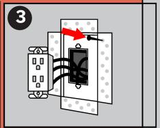
Ensure flange is flat to the wall. Use drywall screws to fasten as needed.
