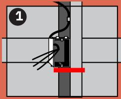
Ensure the receptacle box is installed flush to the studs.
