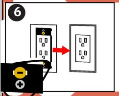
Fasten the screwless wall plate frame and snap on wall plate.
