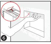
Maintenance post installation can be done through the concealed hinge doors.
