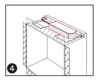
Connect the solderless clamp to the LED Strip, and attach the converter.
