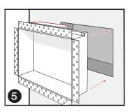
Lay the converter along the top support. Dryfit and connect power.
