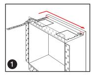
Line LED light strip along the inner top channel. Strip should not exceed channel width of ½ inch.
