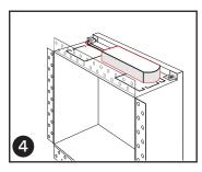
Connect the solderless clamp to the LED Strip, and attach the converter.
