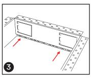
Use adhesive to secure the LED strip to the roof of the channel.
