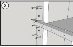
Use provided screws to fasten plates to substrate.
