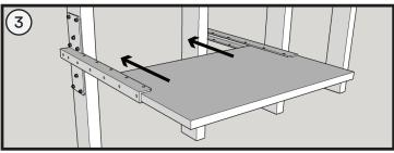
Slide in structural board. Must fit snug with minimal movement.
