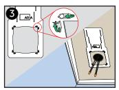
Optional: Use **Smash Plate** as guide. Secure to ceiling using pins as a stamp.
