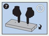
Hold in place and flip **Tray**. Apply even pressure until surface material lies flat with the rim of **Tray**. Leave to cure.
