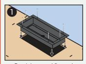
Drop in base on subfloor and fasten with wood screws.
